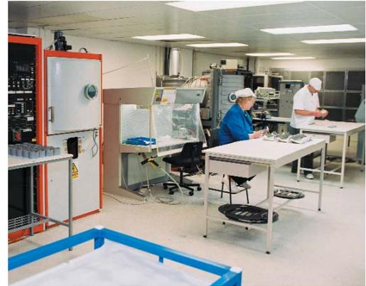
Thin film coatings are applied using high vacuum techniques where materials such as oxides, fluorides and very pure metals are heated by resistive or electron beam methods until they evaporate and deposit onto colder surfaces. Deposition is controlled very precisely to give the required effect for each application and can require from one to over 160 layers of material.
